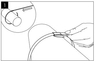
Thread seal in the strap as shown. Bend end of band under seal.
