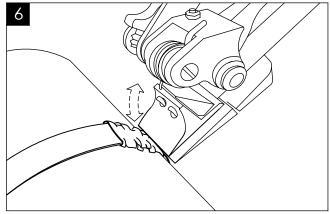
Bend the whole tool forward over the seal and back again a few times to break the strap.
