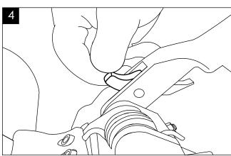
When desired tension is reached, push the handle pawl down to lower the handle.
