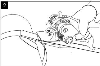
Squeeze the handle down to the base and slide tool onto top strap, feeding strap under feedwheel. Push the breaker nose against seal.
