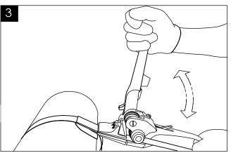
Hold the tool and strap with your left hand and move the handle forward and backward until desired tension is reached.
