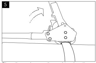
Place the sealer over the seal to crimp the seal.
