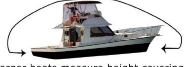
Larger boats measure height covering arches. Remove antenaes
