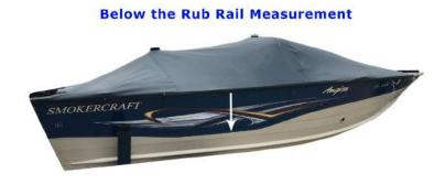
Last, figure out your tucking and fusing measurement. This accounts for the extra material that will be used to tuck the shrink wrap edges under the strap and heat weld the shrink back to itself. Add 6"-1' per side.
