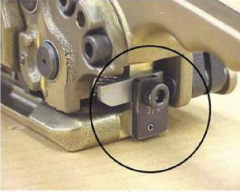
THE STRAP DEFLECTOR IS INSTALLED BEHIND THE BACK GUIDE.
