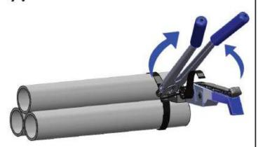
Crimp seal by squeezing sealer handles together.
