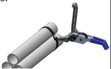
Crank the handle to tension load until taut.
