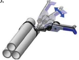
Cut strap by moving tensioner up and down to crease the strap until it snaps off.
