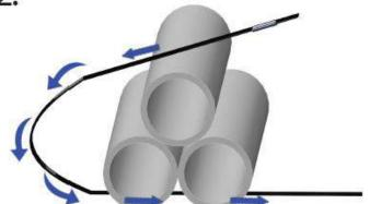
Place steel strap around load. making sure to start by going over the load instead of under.
