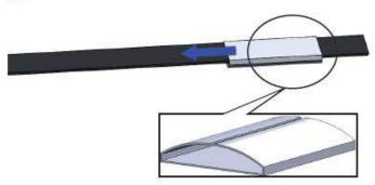
Slide Standard Steel Closed Seal over steel Strap.
