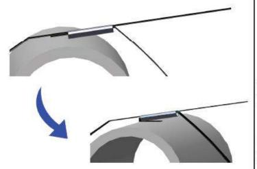
Slide front end of strap under the upper strap and fold the tip of the lower strap under the seal.
