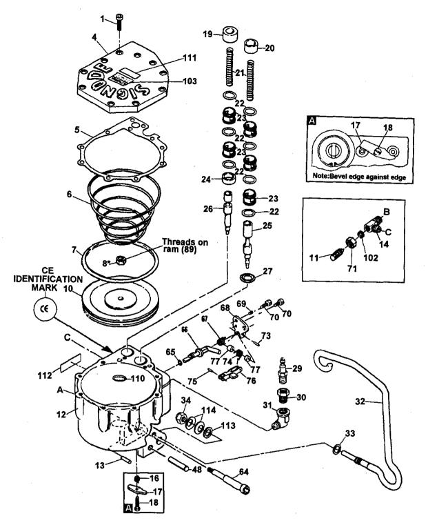
\* Apply one drop of Loctite #242 or equivalent to cleaned parts. Allow 12 hours to set, if possible. Do not apply to small screws or close moving parts as the fluid spreads easily.
